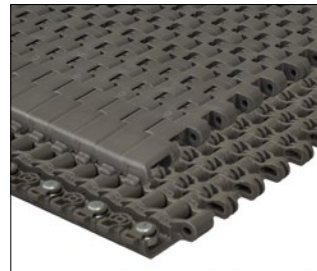
1625 MATTOP CHAIN has a 1.00-inch (25.4 mm) pitch, curved bottom contour and can be used in side-flexing applications
