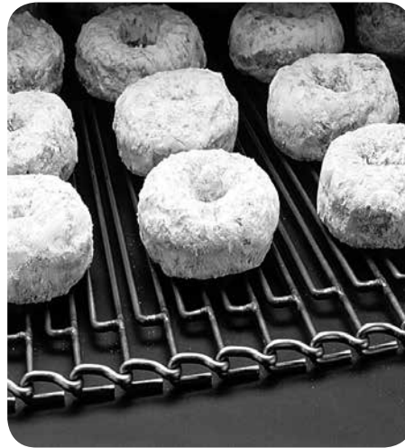
Sani-Grid® with U-bar filler rods.
