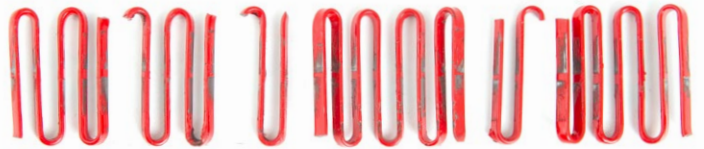
Dodge grid element after 70,000 cycles
