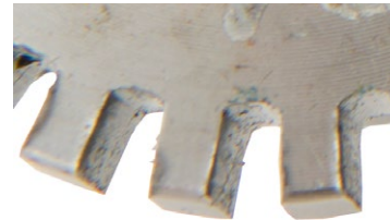
Competitive hub shows pitting on teeth and burrs on tooth edges from broken grid element.
