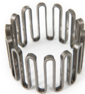
Dodge grid element after 70,000 cycles
