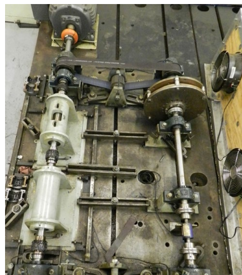
Operating under misalignment test stand
