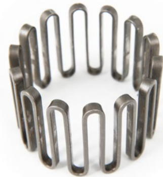
Falk® grid element after 400,000 cycles
