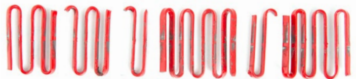
Dodge®* grid element after 70,000 cycles
