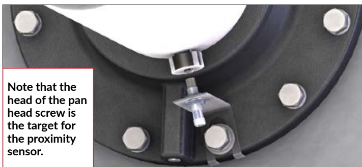
Figure 4 – Finished cylindrical sensor assembly showing bracket legs bent to resist rotation of the bracket during fastener torqueing
