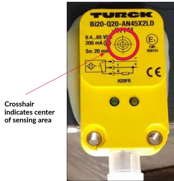
Figure 11 – Flat proximity sensor
