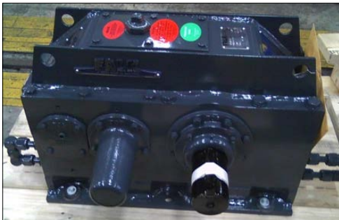
Figure 22 – A and Y units without rounded section at low speed end
