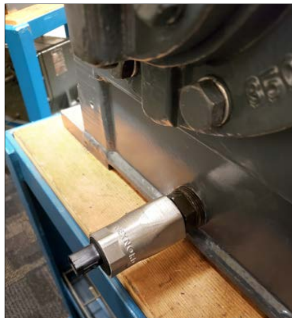
Figure 29 – Assembled and wired oil quality sensor
