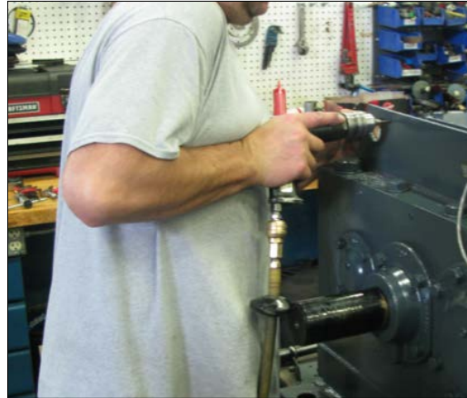
Figure 24 – Hole drilled for Andon light bracket
