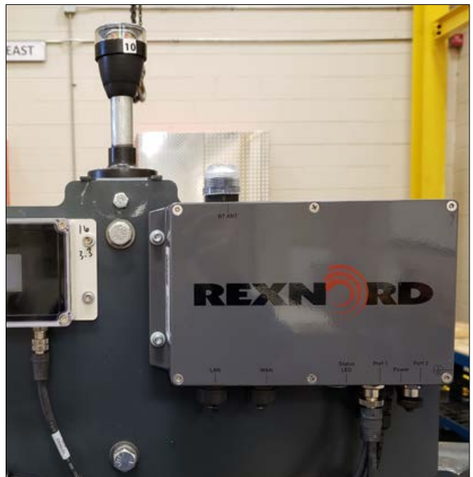
Figure 26 – Assembled andon light mounted on edge mounting plate
