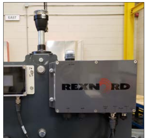
Figure 33 – Assembled andon light mounted on edge mounting plate
