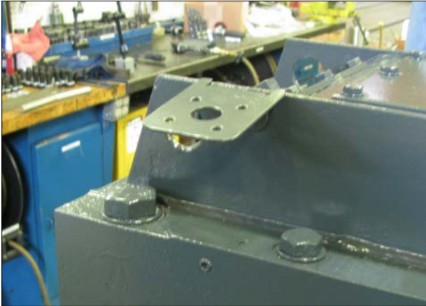
Figure 23 – Andon light bracket positioned near lifting hole
