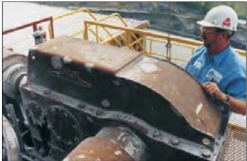
Figure 21 – Y units with sloped and rounded section near low speed end
