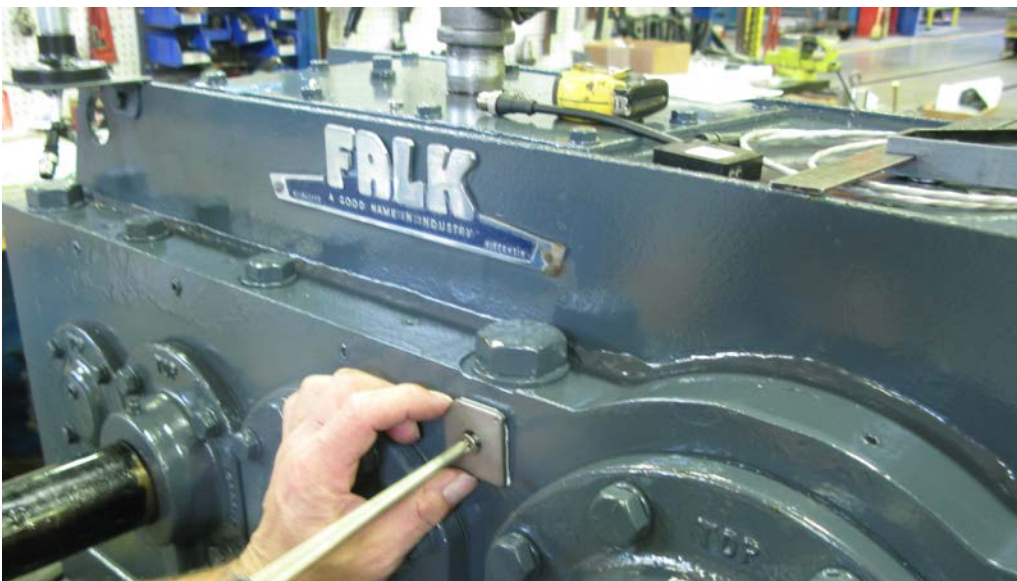
Figure 18 – Bolting vibration sensor mounting plate to housing cover wall
